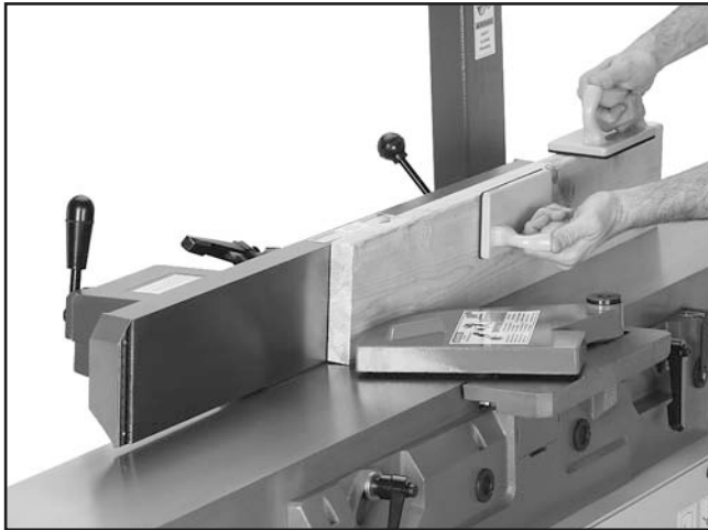
Figure 27. Example of edge jointing operation.
